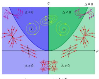
$\frac{\mathrm{d}x}{\mathrm{d}t} = Ax + By \qquad \begin{array}{l} p = A + D \\ q = AD - BC \end{array}$   $\frac{\mathrm{d}y}{\mathrm{d}t} = Cx + Dy \qquad \Delta = p^2 - 4q$
