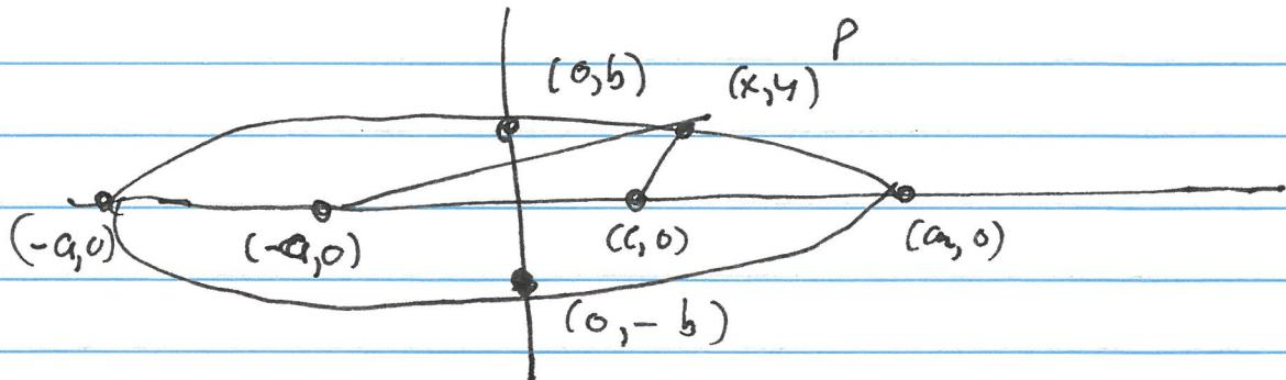
$$(a, 0) \quad \text{DISTANCE from } (c, 0) + \text{DISTANCE from } (-c, 0) \\ = (a - c) + (a - (-c)) = a - c + a \\ = 2a$$
